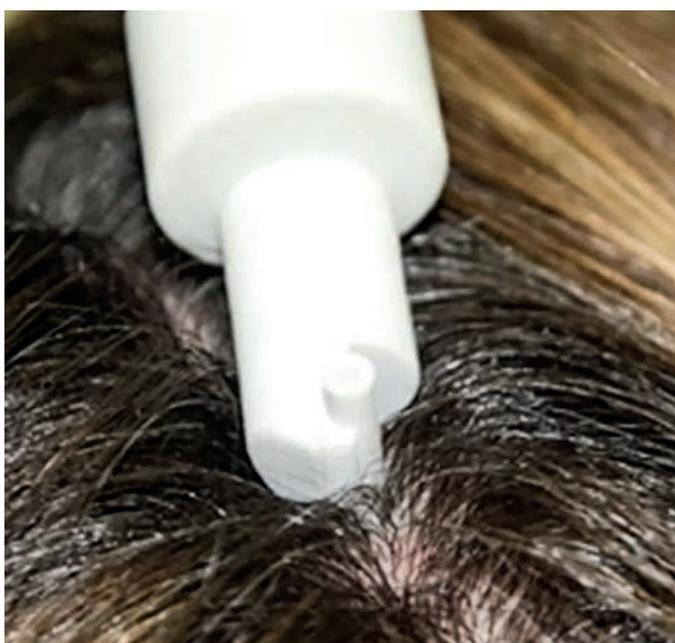
Image 6: Tewameter® Nano, especially developed for TEWL measurements on small and difficult to reach surfaces.
