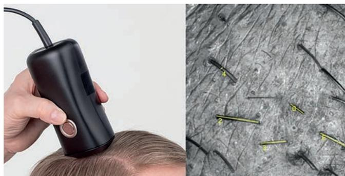
Image 8: Hair length/thickness measurements in mm with the Visioscan® VC 20plus
