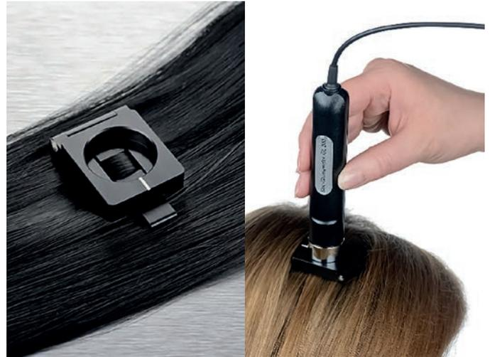
Image 3: Glossymeter and Colorimeter probes used in vivo and ex vivo
